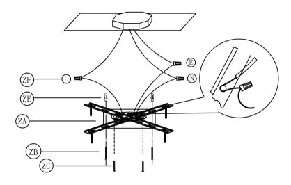
1. Drill two holes on the ceiling and put the plastic anchor screw(ZE) into the holes(If the wall is wood made, this step can be ignored); 2. Attach the Bracket (ZA) to the Junction Box with two screws(ZC).
